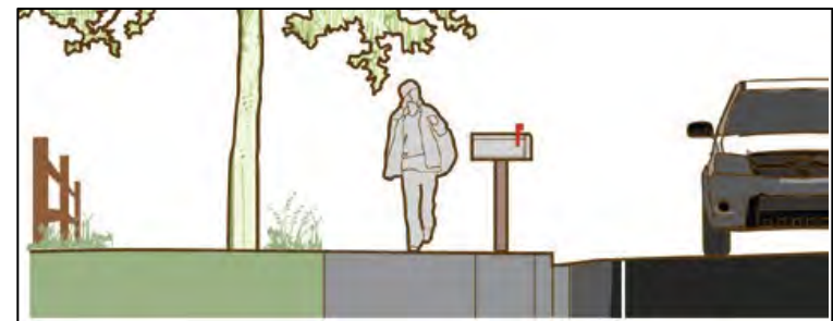
Preferred and alternative sidewalk locations (FHWA Small Town Guide, p. 4-21)
